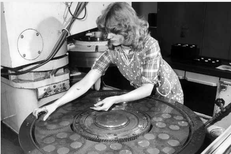
An employee of VEB Spurenmateriale Freiberg manually loads a lapping machine with wafers. In this process step the surfaces of the wafers are mechanically smoothed.
