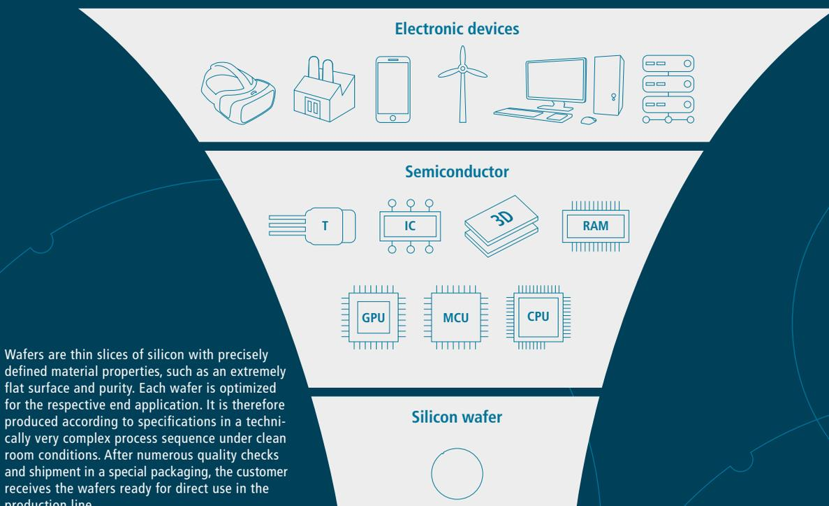
Wafers are thin slices of silicon with precisely defined material properties, such as an extremely flat surface and purity. Each wafer is optimized for the respective end application. It is therefore produced according to specifications in a technically very complex process sequence under clean room conditions. After numerous quality checks and shipment in a special packaging, the customer receives the wafers ready for direct use in the production line.
